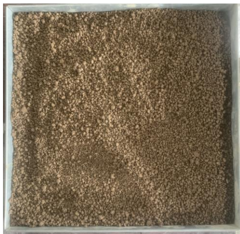
Fig. 6. Compost used in concrete production
