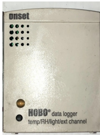
Figure 5. 16 : Thermocouple Data logger type HOBO U12-012 (source: Auteur, 2020).
