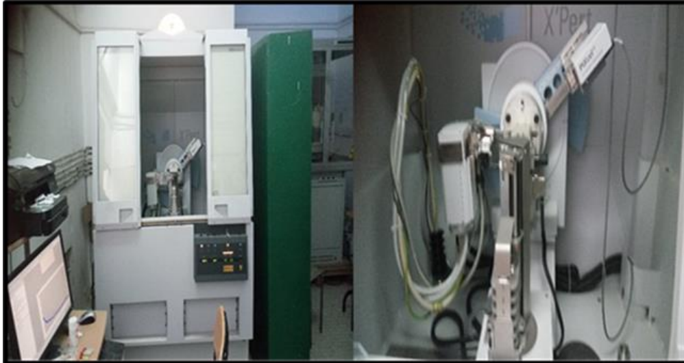
Figure 3.13 Panalytical X Pert Pro diffractometer ( \lambda )CuK \alpha = 1,5406 Å (5°-100°).
