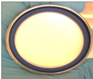
Figure IV-9 : Membrane de microfiltration frontale.
