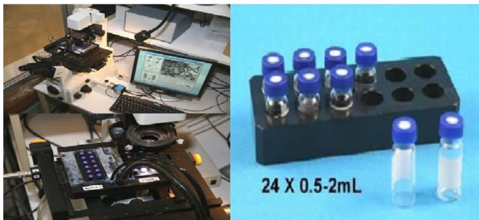
Fig. 2. Images of multi-well, Peltier blocks and corresponding 1 mL vials.
