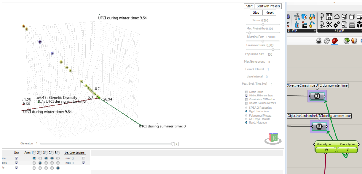
Figure 6.12: Fitness values by Octopus to determine the proper height of new building in Oran (Author, 2018).
