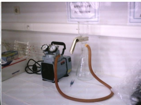
Figure 6: Rampe de filtration
