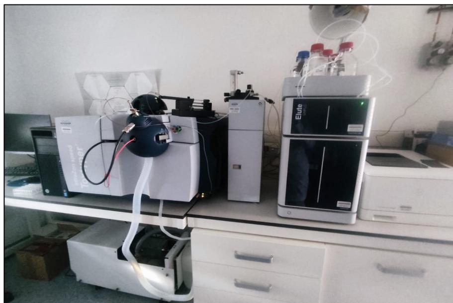
Figure 26. Chromatographe en phase liquide (UPLC) BrukerDaltonics, Bremen, Germany.
