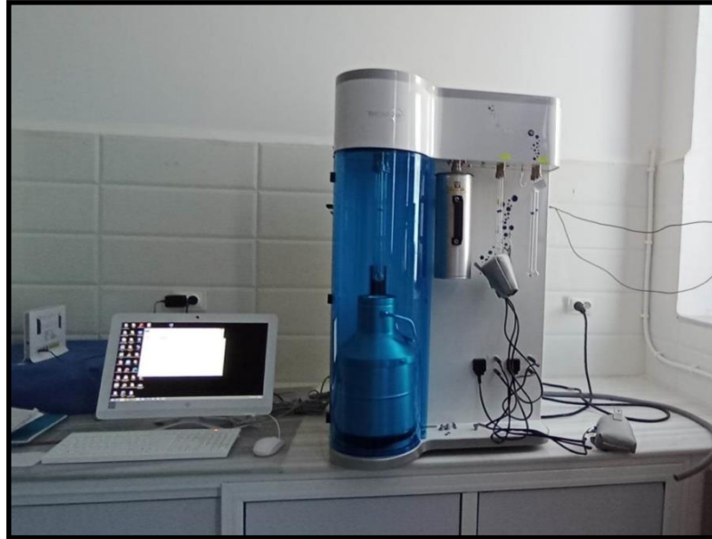
Figure 3.8 :Appareil QUANTACHROME (BET)
