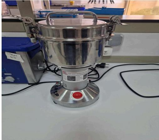
**Figure 3.8** : Broyeur High-Speed Multifunction Grinder.
