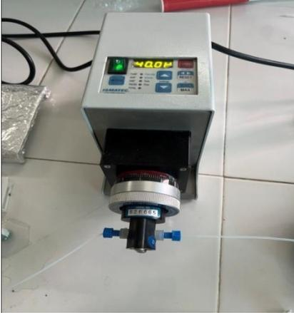
A white peristaltic pump with a digital display showing 400.                          |
