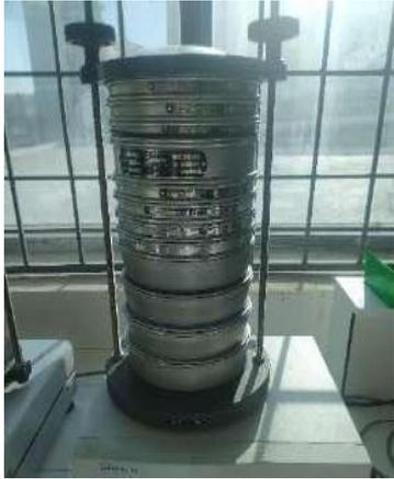
A vertical sieve shaker with multiple stainless steel sieves stacked vertically. |
