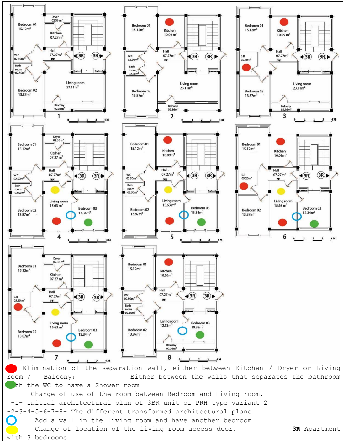
Figure 7. Architectural plans of 3BR unit of the PRH housing program initial architectural plan with the different plans transformed (variant 2)
